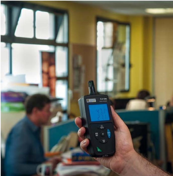
Temperature and Humidity are two other very common measurements taken in a normal work environment, and typically, these two parameters can be found in a single meter called a thermo-hygrometer. With temperature display in Centigrade simultaneous to the measurement and display of relative humidity as a percentage, and some also offering the added capability to display dew point temperature.
