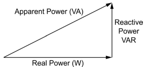
Some electrical equipment used in industrial and commercial buildings requires an amount of Reactive Power in addition to Real or Active Power in order to work effectively. These tend to be items with copper windings in them, especially transformers, motors, induction heaters, arc welders and compressors, etc., even fluorescent lighting.
