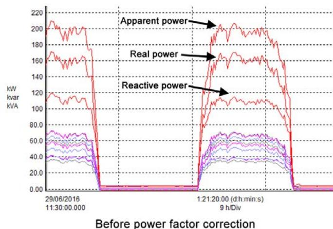
To put that into perspective, a power factor of 0.7 requires approximately 43% more current to do the same thing as an installation with unity power factor. A power factor of 0.5 requires approximately 200% (twice as much) current to handle the same load.
